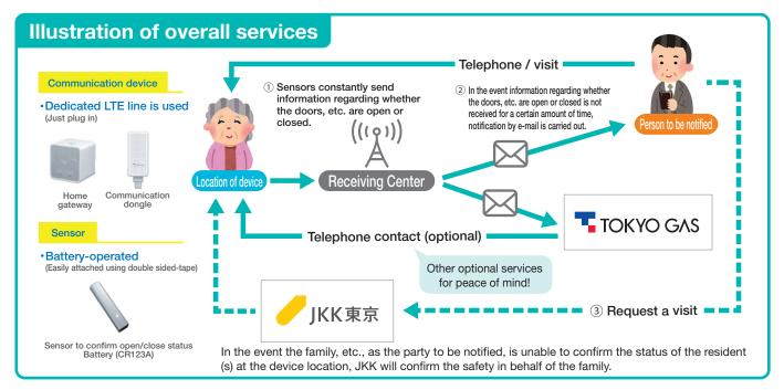
If the door is not opened or closed from 8:00 a.m. the previous day until 7:59 a.m. the current day, the system detects this as an abnormality and will send a notification by email to the pre-set notification address between 8:00 a.m. and 12:00 p.m. of the current day.
