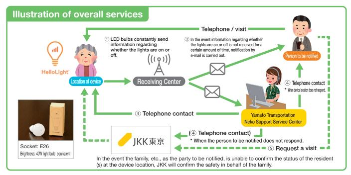
If a light bulb is not turned on or off from 9:00 a.m. the previous day until 8:59 a.m. the current day, the system detects this as an abnormality and will sends an notification by email to the pre-set notification address between 9:00 a.m. and 10:00 a.m. of the current day.
